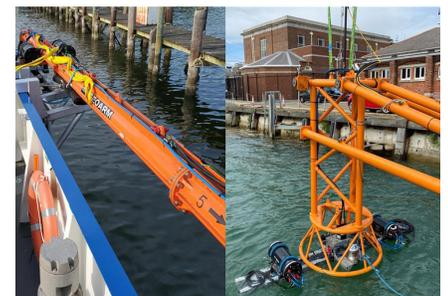
For nearshore applications, the SBI GeoArm and GeoLink can be mounted to vessels and operate in shallow waters up to 15 meters depth in areas such as ports, rivers, and nearshore environments.
