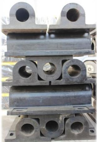
JDO Wing Type Rubber Fenders are developed on the basis of D Type Fenders. They can be fixed with double line anchors which greatly increase the installation stability. Furthermore, their anchoring bolt is bigger than D type so that the anchoring grip is double to D type.
