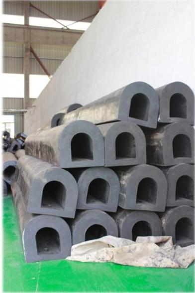
D Fenders can be pre-curved, chamfered and drilled to aid installation at a relatively low cost and can also be cut to the length required. They provide an excellent barrier against damage from all sizes and shapes of vessels. They are ideal for smaller quays and wharves serving fishing boats, tugs, barges and other work craft. D Fenders are also commonly used on pontoons and on inland waterways for lock protection.
