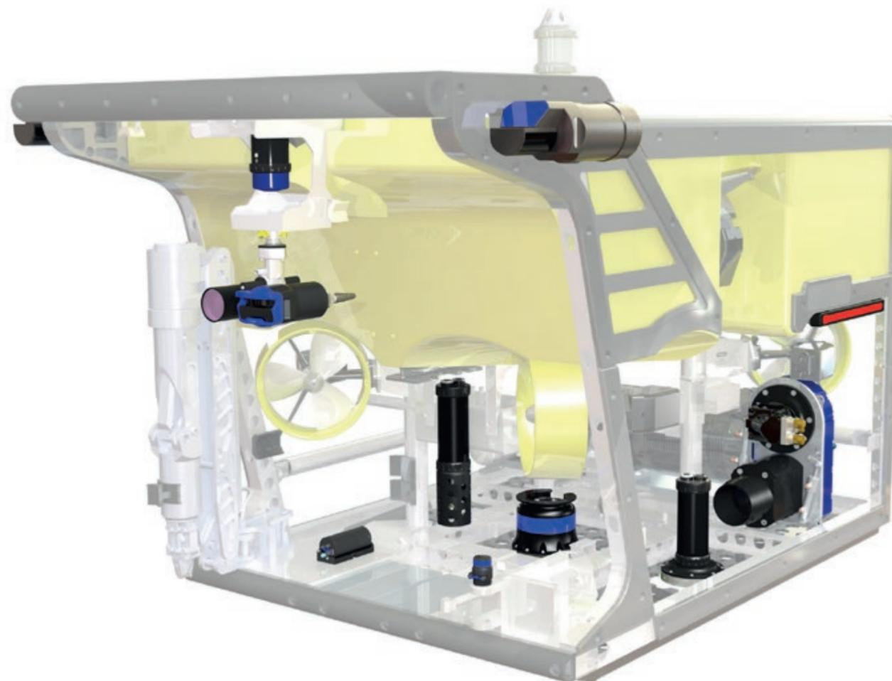
Trittech sensors as installed on a WROV.
