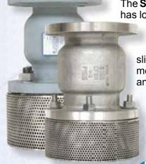
The **Sure Flow Globe Silent Seat Foot Valve** has low head loss through its full ported body area and heavy duty stainless steel basket screening. As pressure increases, the Buna-N Quad Ring is compressed slightly and the disc makes contact with the metal portion of the valve seat, preventing any further compression of the ring. The
