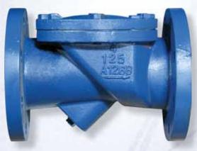
The Elastic Swing Check Valve is suitable for municipal and industrial applications. It is standard with a ductile iron body with ASME Class 125 flanges. The internal body is epoxy coated. The one-piece molded disc has a steel reinforced insert to ensure closure. Plus, while in the open position, it will allow 100% uninterrupted flow. The one-piece disc
