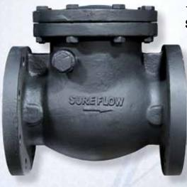
The Sure Flow Horizontal Swing Check Valve has a cast iron body, cover and disc. The valve is provided with a bronze seat ring and bronze disc ring. Bronze, being softer than a cast iron facing, offers a more positive sealing effect than competitors' standard iron
