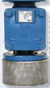
The Elastic Swing Foot Valve is standard with a ductile iron body, ASME Class 125 flanges and is suitable for municipal and industrial applications. The internal body is epoxy coated. Special coatings are available upon request. The one-piece molded disc has a steel reinforced insert to ensure closure, but while in the open position will allow 100% uninterrupted flow. The one-piece disc hinge and flapper can be repaired without
