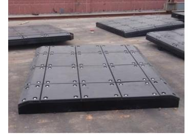
UHMW-PE, Ultra High Molecular Weight Polyethylene, has become the material of choice for facing steel fender panels and where the combination of very high impact and abrasion resistance with low-friction properties is needed. UHMW-PE is the strongest and toughest of all polyethylene grades for marine applications – even outlasting steel as a facing material, and many times better than timber facings.
