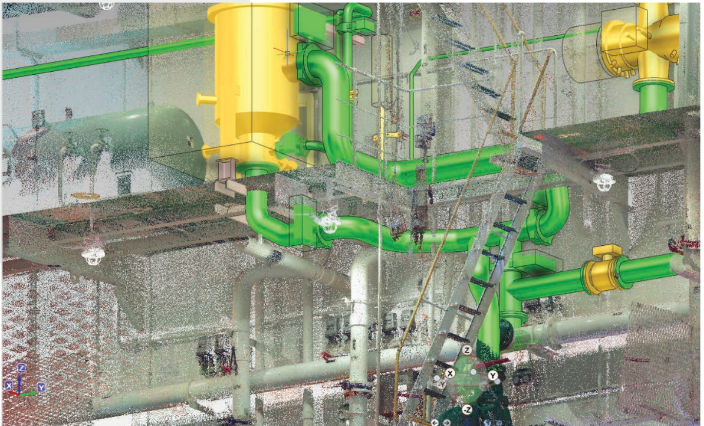
New pipe arrangement for Ballast Water Treatment. Image courtesy of IHB ShipDesign.
